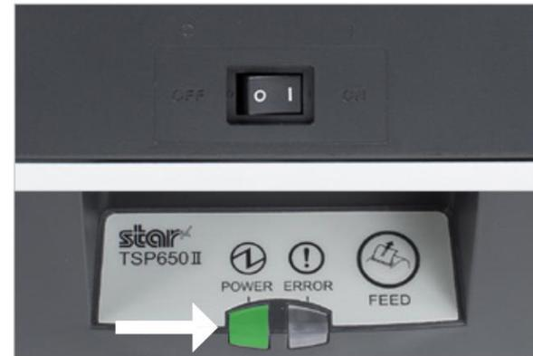
6. Turn Poll Pad Printer ON (switch is on the left side of printer).
